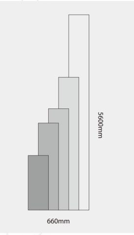
ZX could produce floor with width maximum 660mm, length maximum 5600mm.
